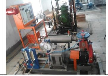
Computerized VCR Diesel engine test rig.
